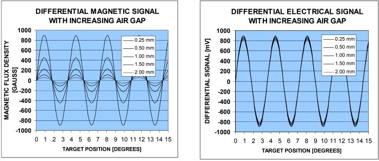
Magnetic Signal with no Amplification
