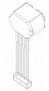
Pin 1: V<sub>CC</sub> Pin 2: V<sub>OUT</sub> Pin 3: Tie to Gnd or Float Pin 4: Gnd
