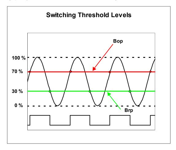
Because the threshold are established dynamically as a percentage of the peak-peak signal, the effect of a baseline shift is minimized. As a result, the effects of offsets induced by tilted or off-center installation are minimized.
