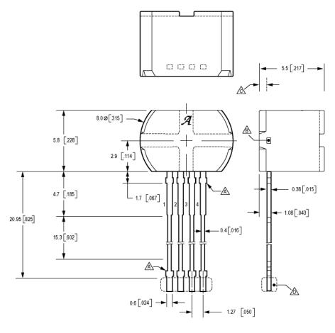
Dimensions in millimeters. Untoleranced dimensions are nominal. U.S. Customary dimensions (in.) in brackets, for reference only A Dambar removal protrusion
