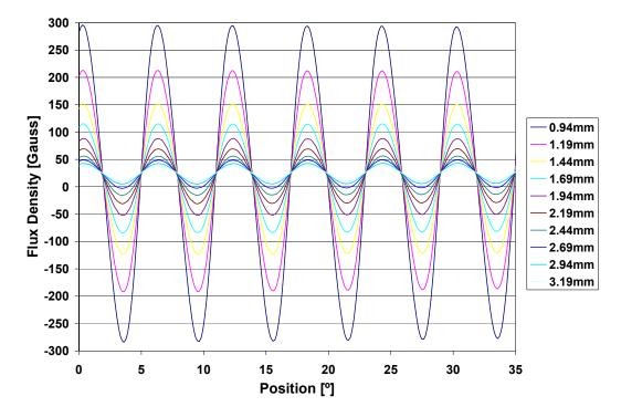
A single curve is distilled from this map data that describes the peak-peak magnetic field versus air gap. Knowing the minimum amount of magnetic flux density that guarantees operation of the sensor, one can determine the maximum operational air gap of the sensor/target system. Referring to the chart below, a minimum required peak-peak signal of 60G corresponds to a maximum air gap of approximately 2.5 mm.
