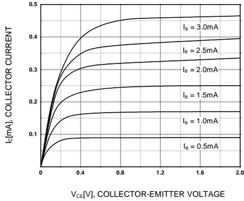
Figure 1. Static Characteristic
